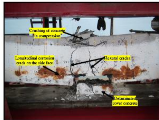
(b) Side view of a corroded RC beam (beam 17) at failure
