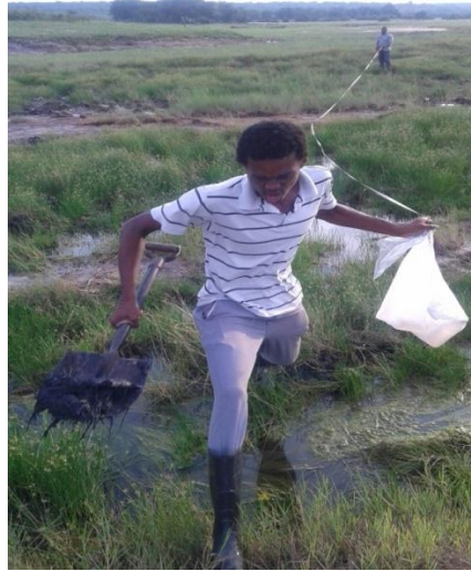
Figure 10. A tape measure used to measure the 50m interval between sampling points.
