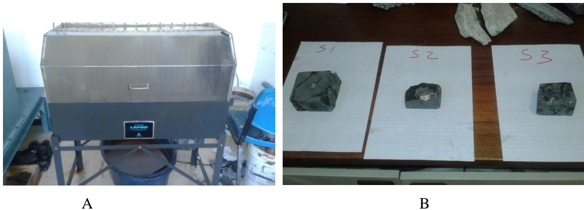
Figure 16. A) The buehlerlapro slab saw 18 was used to remove the weathered part of the rock samples. B) The rock samples being air dried after they were washed with water and soap.
